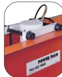
Cylinder is easily moved across width of upper bolster.
