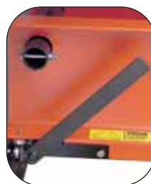
Lever lowers bed for pressing, raises it for rolling.
